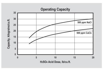
OPERATING CAPACITY — Capacity is based on 500 ppm of stated salt (as CaCO3) with 0% alkalinity, 36 inch bed depth, flow rate of 2 to 4 gpm per cu.ft., and a minimum of 30 minutes chemical injection time. Sulfuric acid concentration must be stepwise when calcium concentration exceeds 20% of total cations. No engineering downgrade has been applied.
